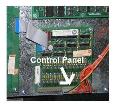
For People with a Sinistar or Blaster with a 49 Way Joystick your adapter harness has an additional harness part that adapts the stock connections from the joystick down to the header connection to hook to the Main PCB.
