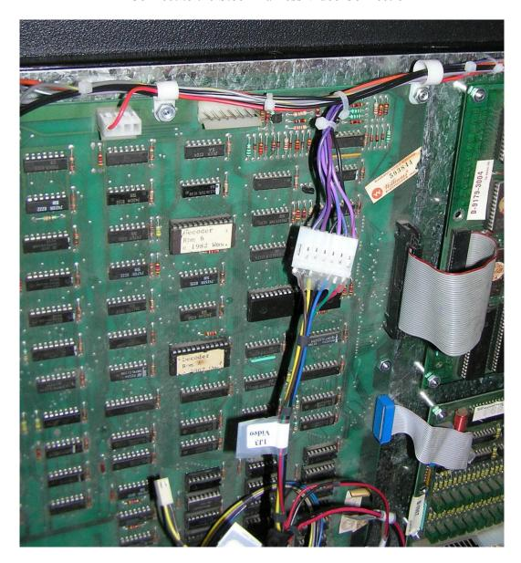
2<sup>nd</sup> connect the H & V Sync Connection to your Jrok Multi-WMS PCB Header. For Reference: V-Sync is the Yellow Colored Wire H-Sync is the Brown Colored Wire
