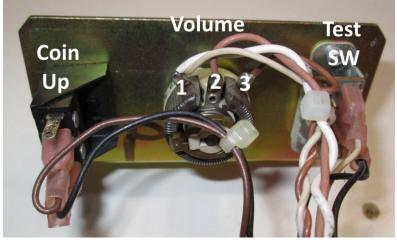
Volume/Credit/Test Plate Brown and Black Wire = Coin Up Switch White and Black Wire = Test Switch Volume Switch 1- Both White Wires (One to Speaker and one to P8 on AR Board 2 – Brown wire from Speaker 3- Brown Wire from AR Board P8
